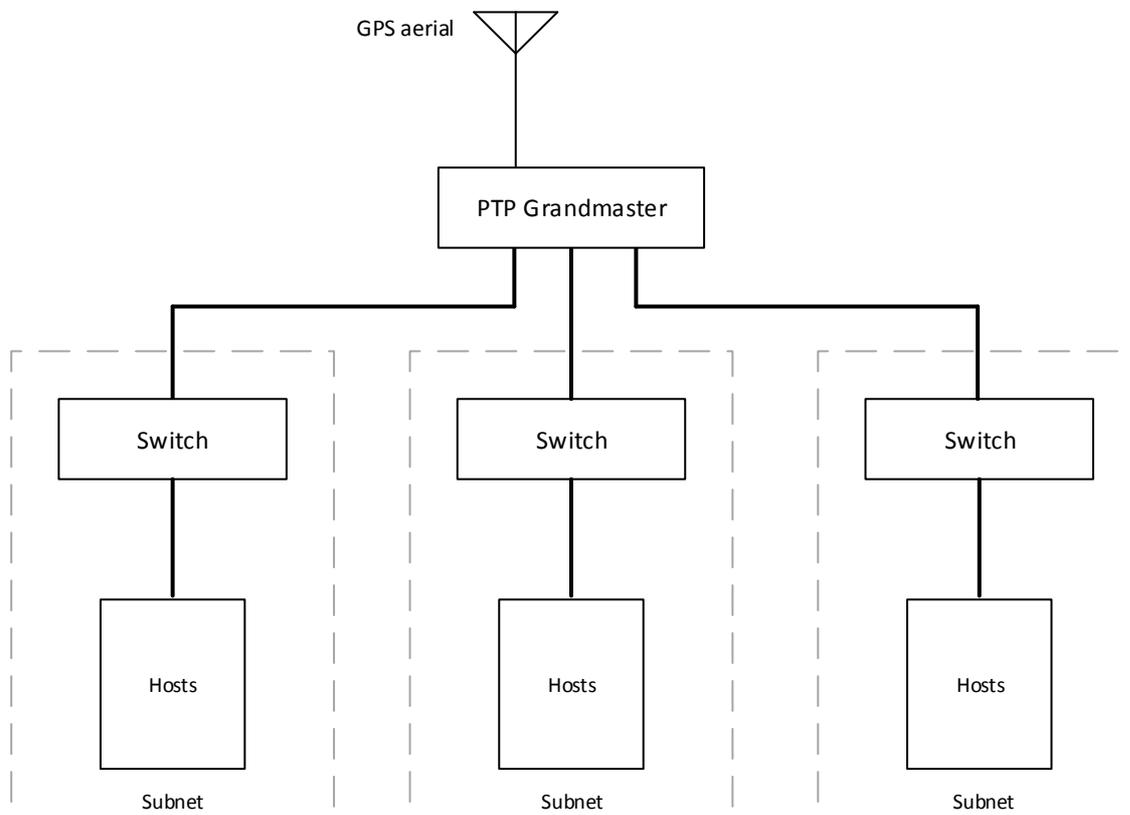
Diagram 3 shows a PTP GM that distributes PTP to multiple boundary clock PTP appliances, each of those is servicing hosts in one subnet.
