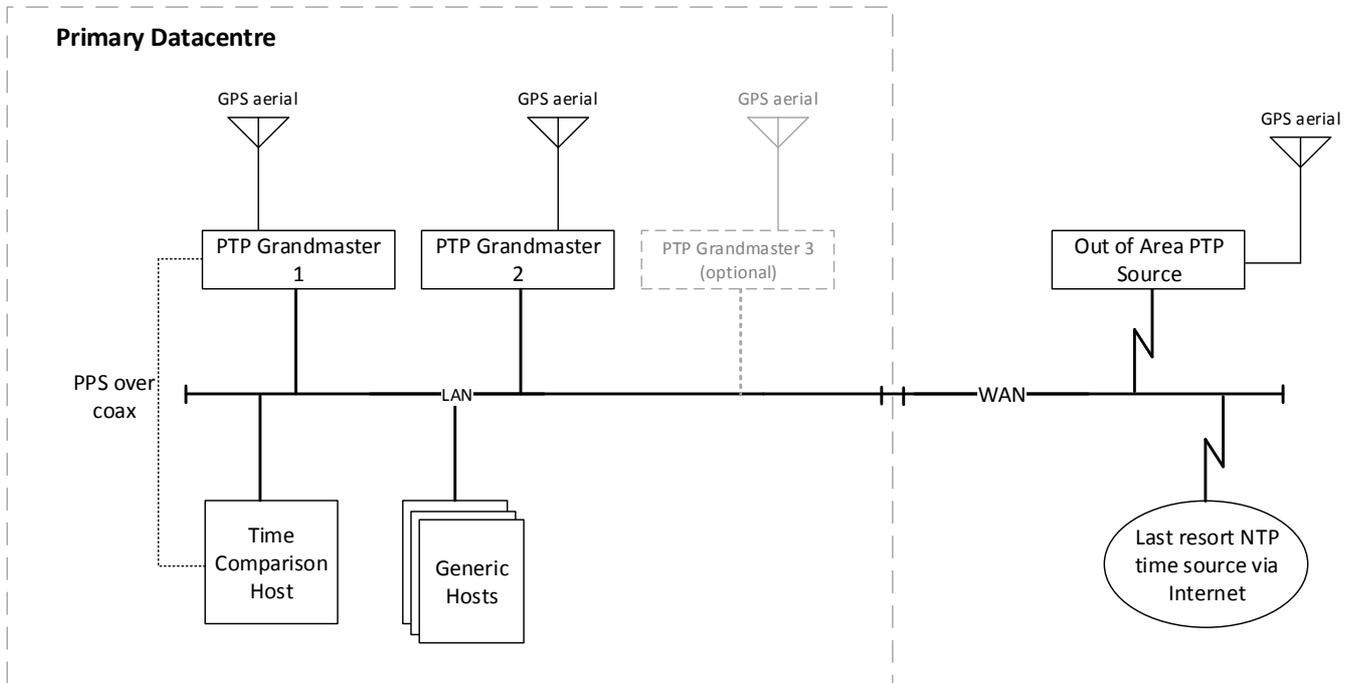
In addition to the design shown in diagram 1, each trading environment has a “Time Comparison Host”. This host continually pulls in time information from multiple sources, compares them to each other and records all deltas for alerting and graphing.
