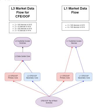
The expected latency advantage of an L1 connection compared to a L3 connection is between 2-4 microseconds. L1 connections will experience less jitter and reduced port-to-port latency (single nanoseconds) when compared to L3 market data connections.
